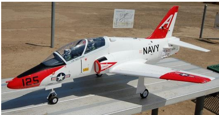
Frank Baker's T-45C Goshawk with flaps, retracts, speed brakes, lights, and tail hook. It has a 90 mm EDF by Free Wing.
