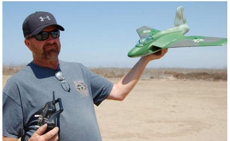
Jeff Denham and his Lippisch Lip-15. It has a 64 mm Electric Ducted Fan (EDF) and runs on 3 cells. This plane was never built by the Germans but was jet powered based on the Me-163 rocket powered Comet.
