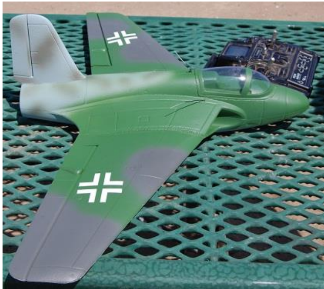
Jeff Denham and his Lippisch Lip-15. It has a 64 mm Electric Ducted Fan (EDF) and runs on 3 cells. This plane was never built by the Germans but was jet powered based on the Me-163 rocket powered Comet.
