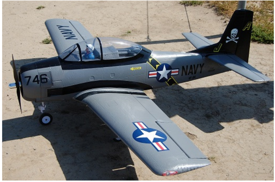
Jerry Smith poses with his T-28 by E-Flite. It has a 5048 size 125 KV motor, 83" span, flaps, retracts, and engine sound system.
