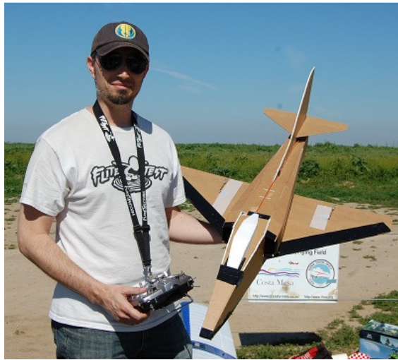
Jerry Smith poses with his T-28 by E-Flite. It has a 5048 size 125 KV motor, 83" span, flaps, retracts, and engine sound system.
