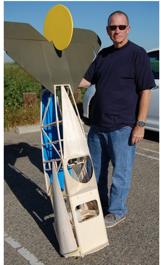
Jerry Smith poses with his T-28 by E-Flite. It has a 5048 size 125 KV motor, 83" span, flaps, retracts, and engine sound system.
