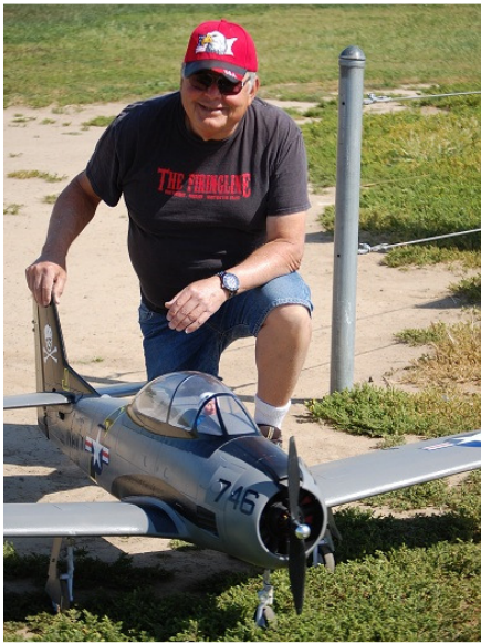
Jerry Smith poses with his T-28 by E-Flite. It has a 5048 size 125 KV motor, 83" span, flaps, retracts, and engine sound system.
