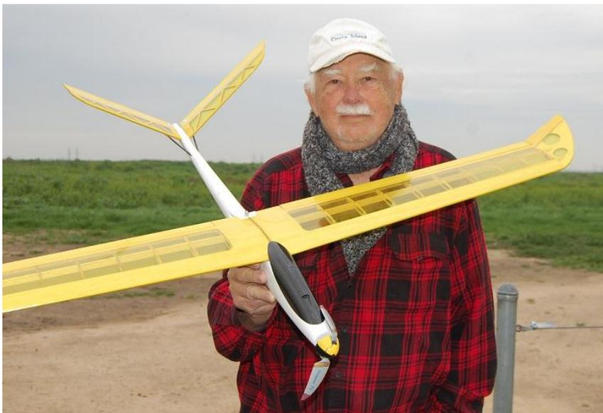
So, Larry Koch solved the problem with his 55" span motor glider, at left. No wheels needed. It is powered with a Mega 16-15-6 motor with a 7x3 folding prop. He uses a 3 cell 1500 mAHr Lipo battery. You can't tell this beauty is 10 years old, below left.
