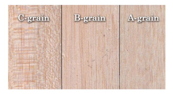
Builders should take note of the different balsa grains. Each grain type has different characteristics and should be used in different applications.
