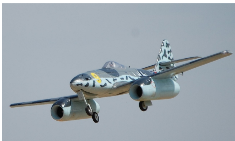
Dave with his Me-262 twin 70 mm EDF, runs on 4 cell 5 AHr batteries. 60 " span from Dynam. Flies very well.
