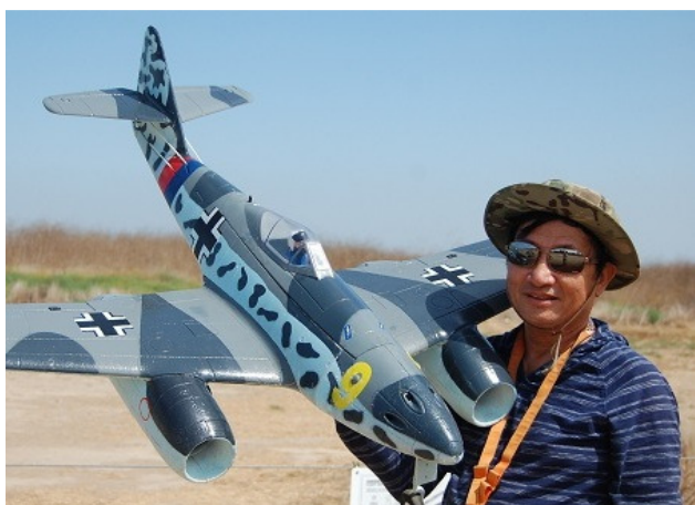
Dave with his Me-262 twin 70 mm EDF, runs on 4 cell 5 AHr batteries. 60 " span from Dynam. Flies very well.
