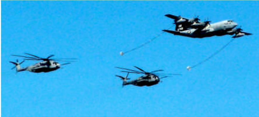
Two Marine helicopters are hooking up for refueling.
