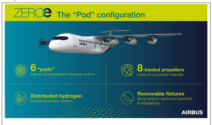
With the move towards electric aviation comes new opportunities to explore what a powertrain looks like, and Airbus is experimenting with a new design that builds entire hydrogen propulsion units, tanks and all, into detachable pods along the wings.
