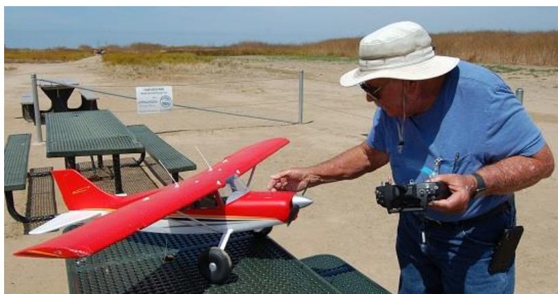
Jim Hanson with his Maule RM-7 bush plane. It is a 60" span Bind-N-Fly from E=Flite, with altimeter and GPS.
