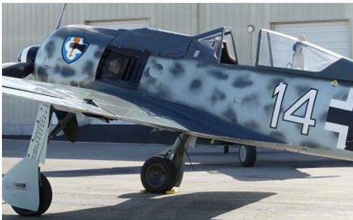
FW-190 rebuilt from actual parts and also new parts made from drawings. Powered with an American Pratt and Whitney engine.
