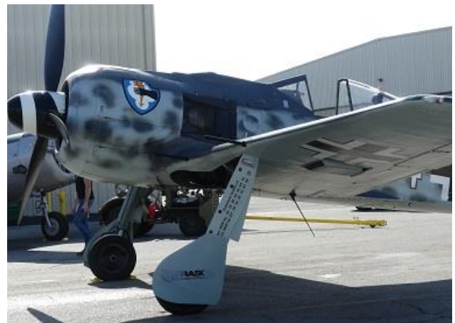
FW-190 rebuilt from actual parts and also new parts made from drawings. Powered with an American Pratt and Whitney engine.
