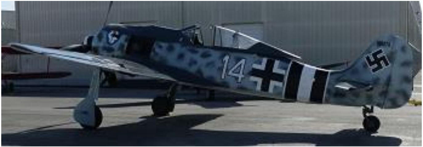
FW-190 rebuilt from actual parts and also new parts made from drawings. Powered with an American Pratt and Whitney engine.
