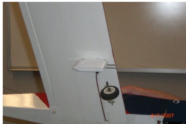
Airspeed and static pitot tubes on bottom of wing.
