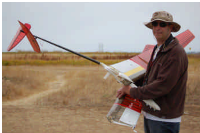
Above, Mike Morjoseph holds the sad remains of his AVA that broke a spar on launch.
