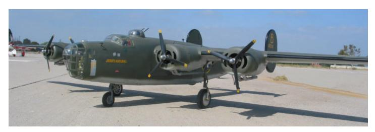
This beautiful lady had four Magnum 61's for power, retractable landing gear, and all the superb detail of a first class scale model. It was built from an American Eagle kit. The pre-flight warm up was a major task, as each engine had to be individually tuned to maximum power and matched RPM using a tachometer.
