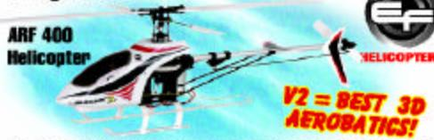
V2 Features: new, strong, durable, toothed belt system for driving the tail rotor. New, wider landing gear, updated body style, ball linkages, new tail rotor servo position (tail boom), extended battery tray makes it easier to install Li-Po batteries.
